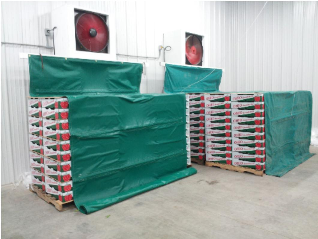
[Polter's Berry Farm](#) in Ohio uses this forced air cooling system. The forced air cooler draws cool air in from the sides across the fruit and out through the exhaust fan.
